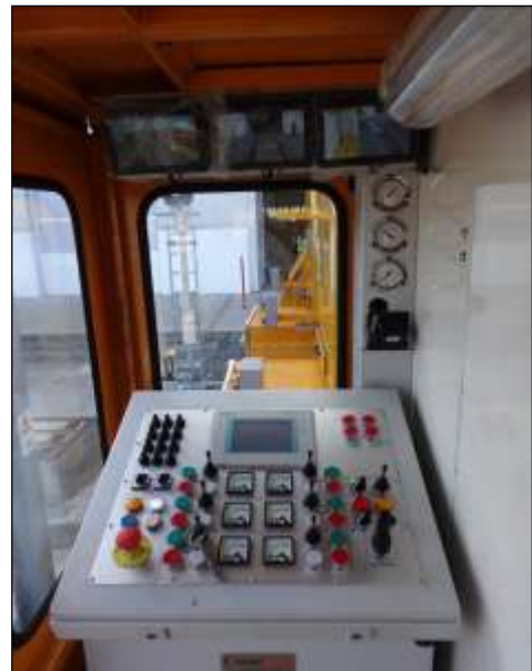
PLC main control panel
